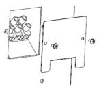
**Step 2:** Connect the Battery Cable to the battery input Terminal Block and ensure the polarity is right, then retighten the Block Cover.
