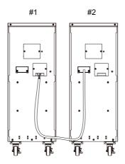
**Step 5:** Rotate the battery cable retention bracket and tighten the screws to fix battery cable.
