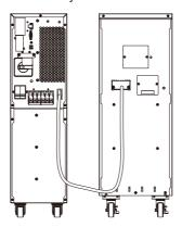
**Step4:** Rotate the battery cable retention bracket and tighten the screws to fix battery cable.
