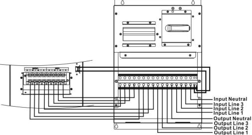
**NOTE:** Make sure that the wires are connected tightly with the terminals. Put the terminal block cover back to the rear panel.
