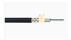
Structure: 0.25MM color fiber\*12/24+ Aramid yarn +inner jacket +stainless steel tube+ Aramid yarn+ outer jacket
