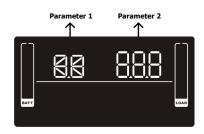
There are three parameters to set up the UPS. Parameter 1: It's for program alternatives. Refer to below table.
