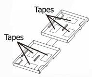
Step 3: Put assembled battery packs on one side of plastic shells as below chart.
