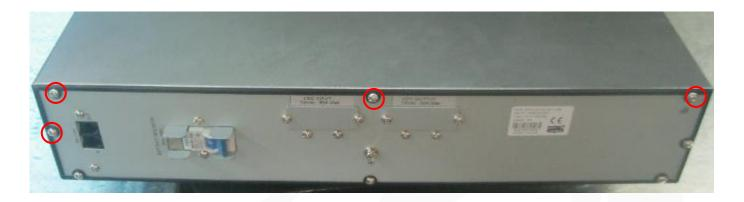
2. Lock the both side screws of the outer cover as shown below: 38-000029-XXG\*11 Torsion:
