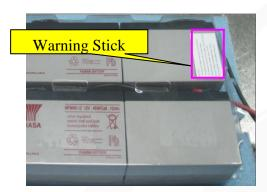
2. As shown left: Put on the warning stick (37-000031-XXG) onto the battery (text facing up)
