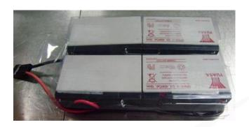
1.As shown left: get the batteries stuck onto the double-side tap on the previous isolation tray
