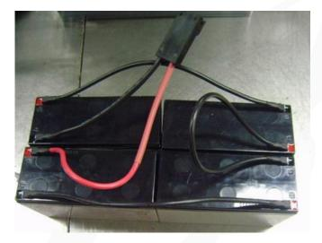
2. As shown left: get 4 batteries in serial connection
