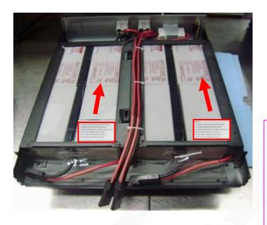
1.As shown both of two: Push the assembled battery bank into the case following the instructed direction (the red arrow)
