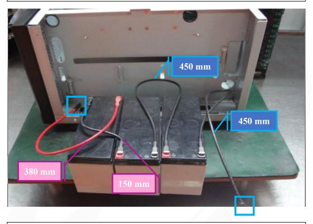
Organize the batteries as shown below. Use the protective plastic to avoid sharp edges damaging the wires. Fasten the batteries with the fixing plate.
