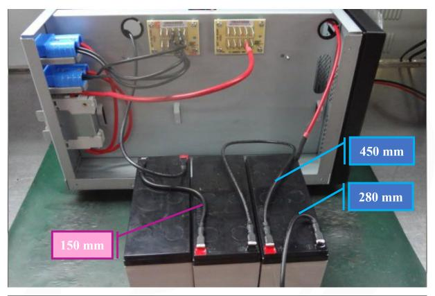
Organize the batteries as shown below. Use the protective plastic to avoid sharp edges damaging the wires. Fasten the batteries with the fixing plate.
