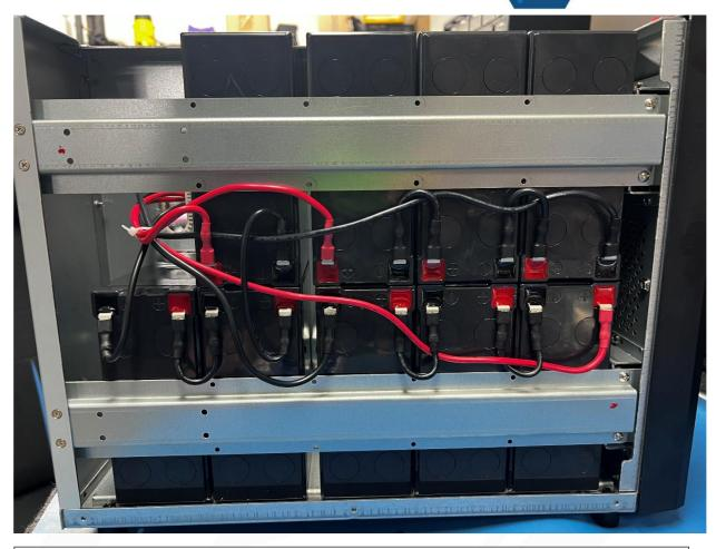
Please use the in-package protective plastic to avoid sharp edges cutting through the cables. Organize the cables as shown in the picture.
