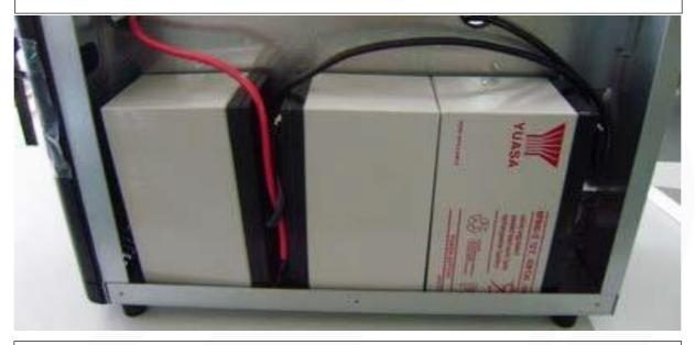
Please use the in-package protective plastic to avoid sharp edges cutting through the cables. Organize the cables as shown in the picture, and place and screw the fixing plate on top of the batteries.
