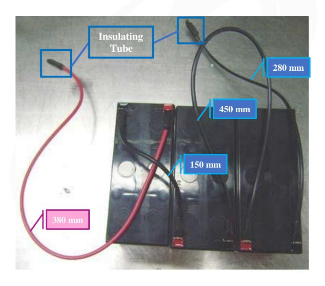
Put the three batteries in order as shown in the picture.
