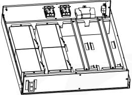
**Note:** To install the second branch of batteries, repeat the same procedure on the right side of battery box.
