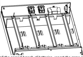
**Note:** To install the second branch of batteries, repeat the same procedure on the battery fixing plate on the right side of battery box.
