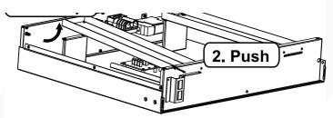
**Note:** To install the second branch of batteries, repeat the same procedure on the battery fixing plate on the right side of battery box
