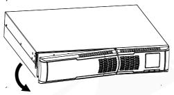
Step 3: Remove the fixed part of the front panel by removing 2 screw present.
