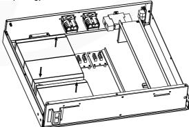
**Note:** To install the second branch of batteries, repeat the same procedure on the right side of battery box.
