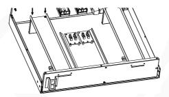
Pull up first and then push the battery fixing plate.
