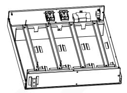
**Note:** To install the second branch of batteries, repeat the same procedure on the battery fixing plate on the right side of battery box.
