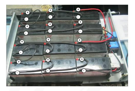
**Note:** The cable connection from external battery connector to PCB is already present inside the battery box. All the other cable connection should be followed by wiring diagram.
