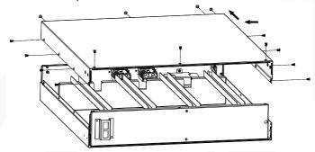
Step 5: Once the battery box is opened, remove the battery fixing plate present on the left side of the battery box by unscrewing the 2 screws present.
