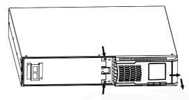
Step 4: Remove the metal top cover of the battery box by unscrewing 8 screws present on the two sides (4 on the right side and 4 on the left side), 3 screws on the top and 4 screws on the back side.
