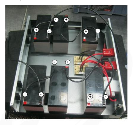
**Note:** The cable connection from external battery connector to PCB is already present inside the battery box. All the other cable connection should be followed by wiring diagram.
