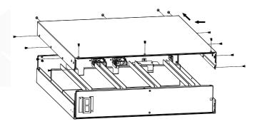
Step 5: Once battery box is opened, remove the battery fixing plate present on the left side of the battery box by unscrewing the 2 screws present.
