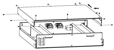
Step 5: Once battery box is opened, remove the battery fixing plate present on the left side by unscrewing 2 screws present.
