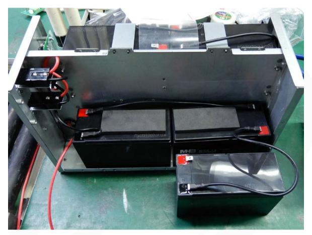
**Step 5**: Lay up the batteries follow the picture and set up the metal support to fix the batteries.
