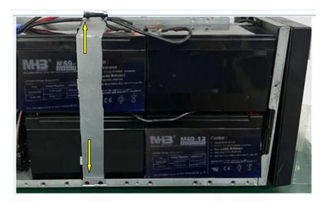
Step 3: Stack the batteries, connect the two batteries with a short black wire, and then connect the red wire of fuse board; Install the insulating sheet on the upper battery terminal
