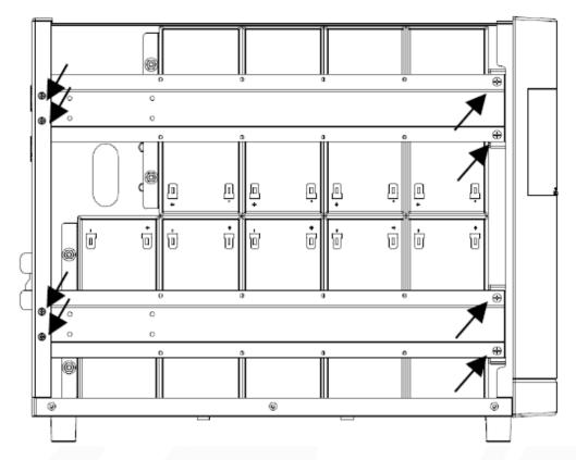
Step 7: Put metal top cover back to the unit and secure it with screws.
