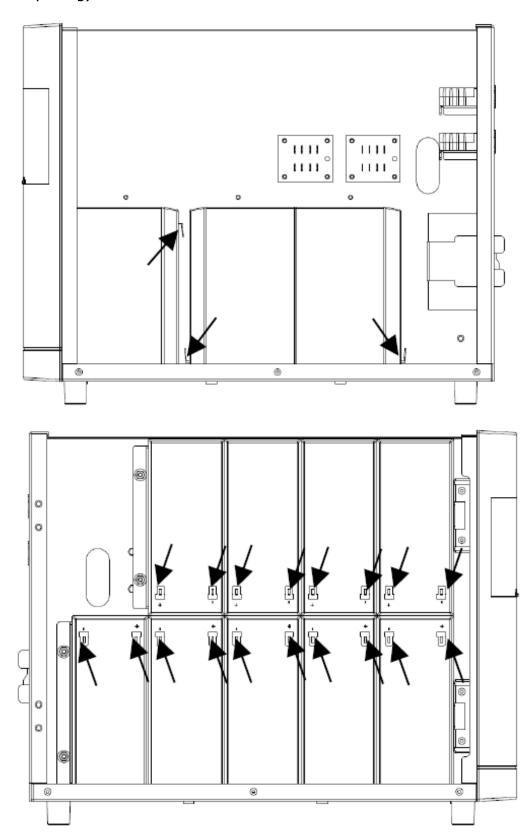
Step 5: Connecting the batteries following the wiring diagram.
