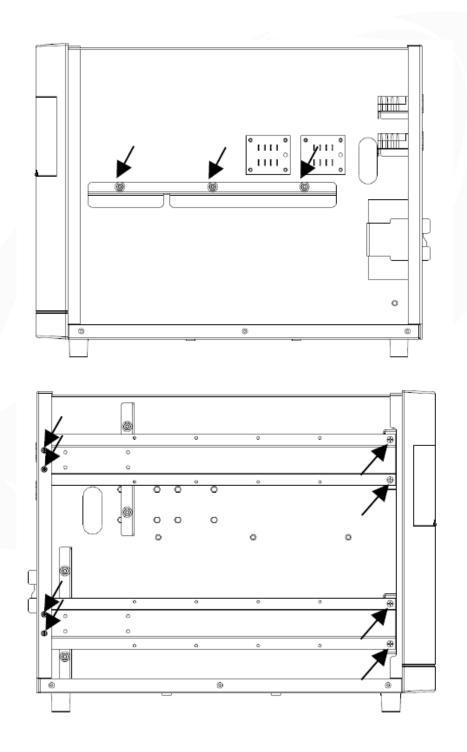
Step 4: Now, it is possible to put all batteries in battery pack following the picture below (in the following drawing is indicated the fasten positions for the correct batteries placing).
