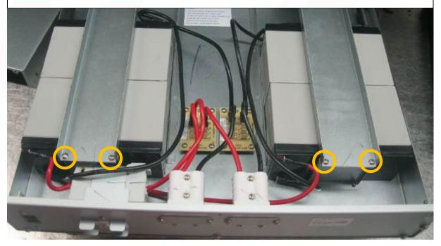
*Abbildung 3: Lock the guard plates*
