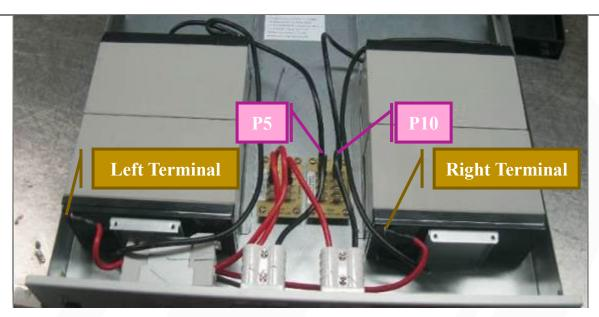
Abbildung 2: Terminal and PCB connections
