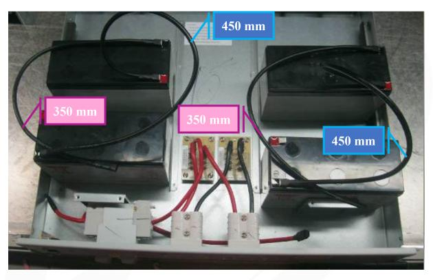
Abbildung 1: Cable lengths and initial connections
